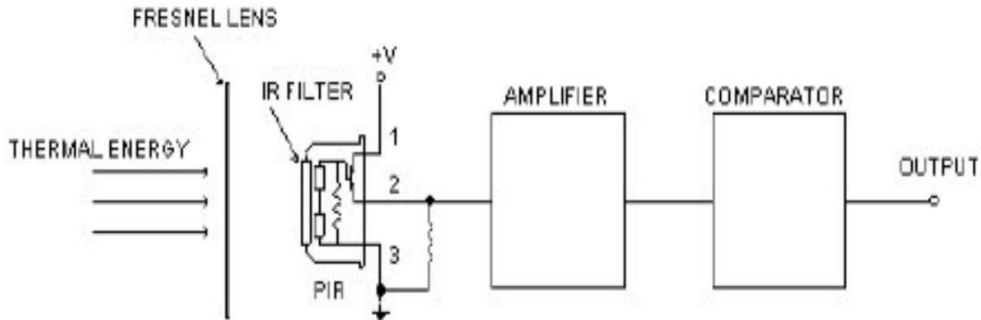
Figure 3. Internal structure of PIR sensor.
