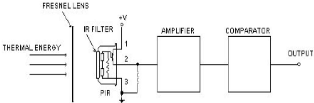
Figure 3. Internal structure of PIR sensor.
